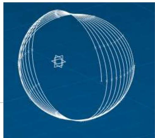
The intent was to create a 5 second trace of the tip of one blade when the fan is turning at 120 rpm and the body of the fan rotating on its axis at a speed of 2 rpm, using the skeleton methodology, linking designer models with product level publications.
